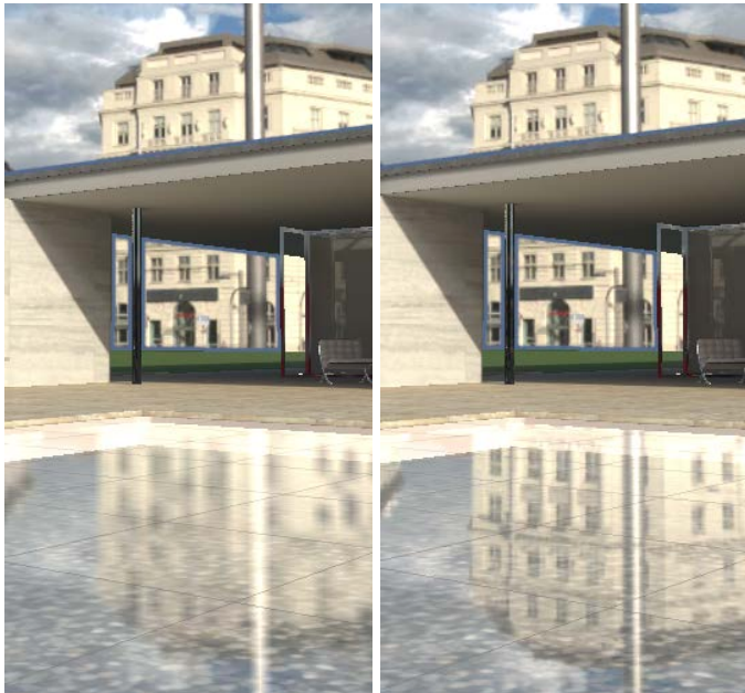
Left: The standard resolution of 128 is used for the environment reflection. Right: The increased resolution of 512 means that a cube map of 6 images with 512x512 pixels is used for the reflection.
