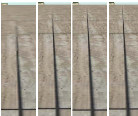
From left to right: 1, 4, 8 & 16 Aniso(tropic) Level. The number means how many texels (= texture image pixels) are involved in creating the final pixel displayed. The more are, the more expensive it is in terms of performance.
