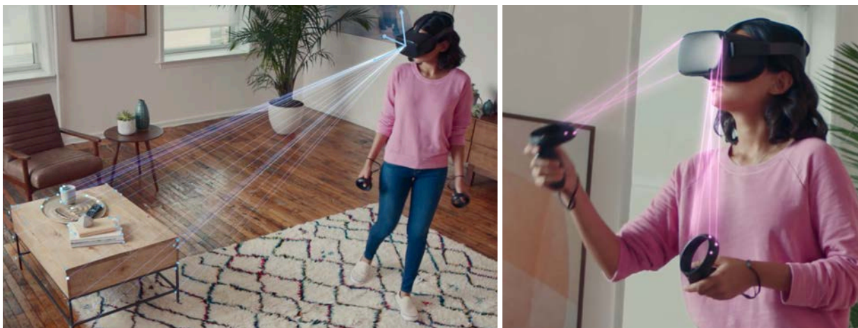
The Quest uses an inside-out 6DOF tracking system named Oculus Insight . The system relies on four wide-angle cameras mounted at each corner of the headset to track the headset and its controllers in 3D space. These cameras can also detect your hands so you can use the headset without controllers.
